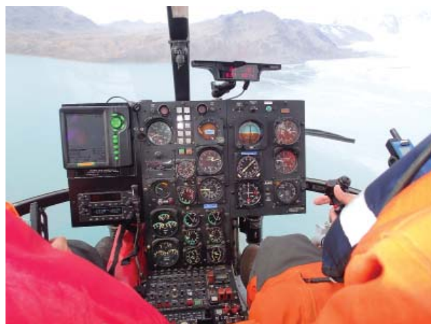
Fig. 4 TracMap TM GPS guidance equipment fitted to South Georgia Heritage Trust aircraft, 2015.
